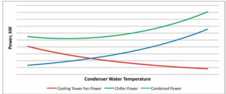
Figure 2: Cooling tower power consumption VS water temperature
